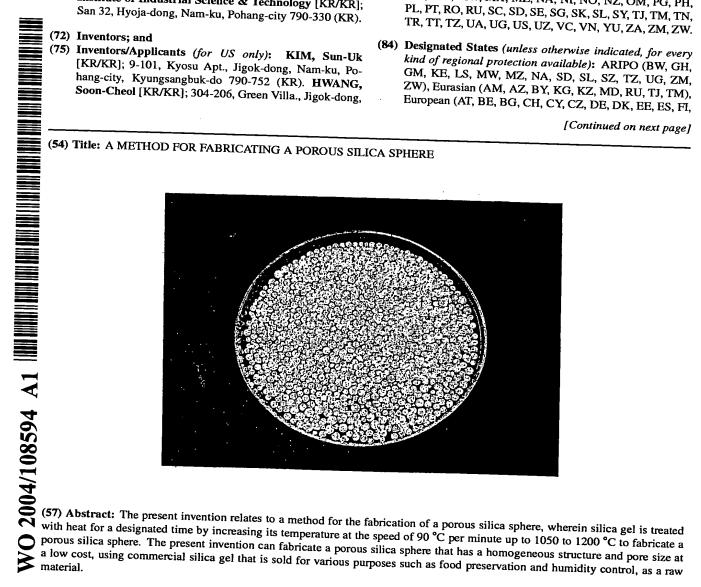
porous silica sphere. The present invention can fabricate a porous silica sphere that has a homogeneous structure and pore size at a low cost, using commercial silica gel that is sold for various purposes such as food preservation and humidity control, as a raw material.
